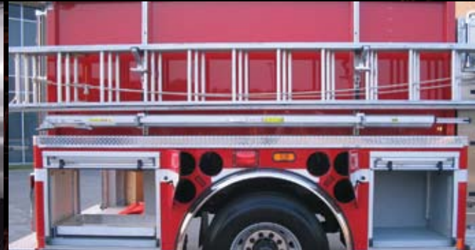
Traditional ladder storage on right side
